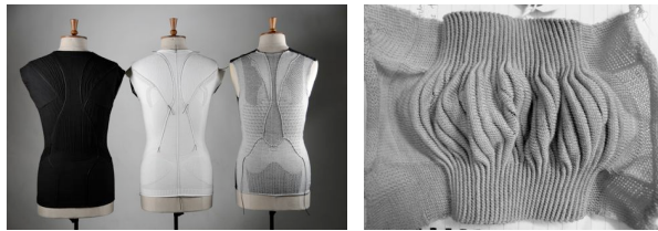
figure 1. Integration of rubber cord stretch sensor into (l to r) aesthetic embroidery, knit and weave structures. Figure 2. custom knit sensor using Bekaert steel yarn.
