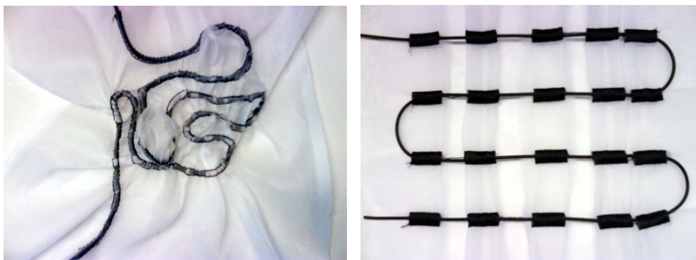
figure 4 Tina Downes experimental embroidery samples incorporating rubber cord stretch sensor
