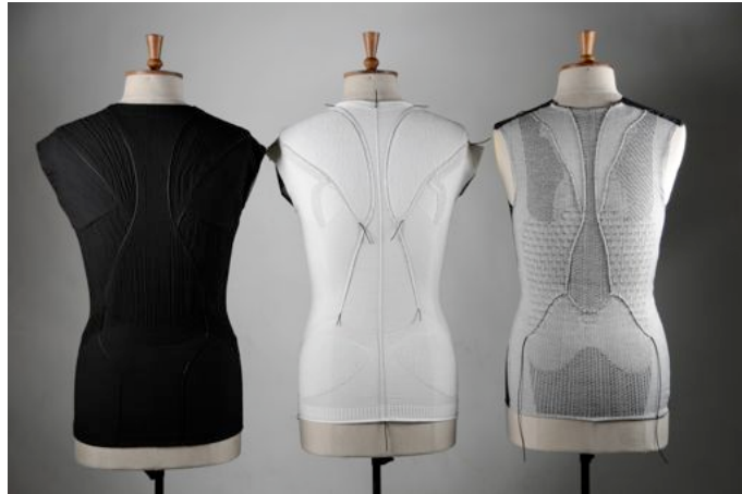
Figure 1 the backs with Merlin stretch sensor l to r: embroidered, knitted, woven
