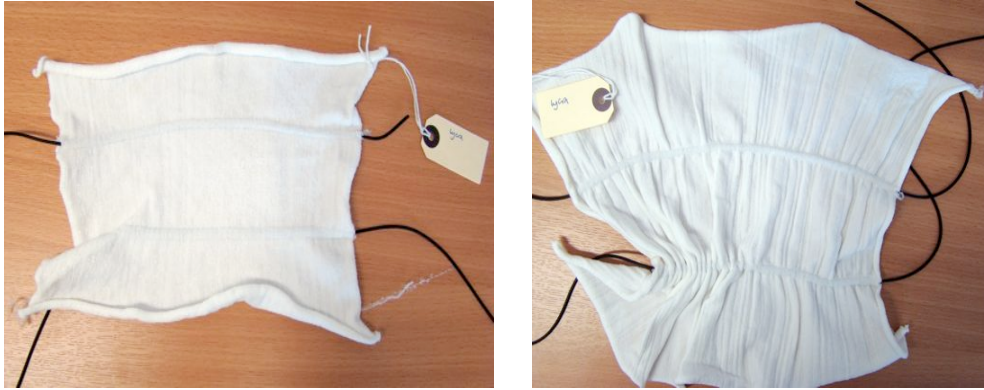
Figure VI: Embedding - Lycra knit with channels threaded flat and ruched
