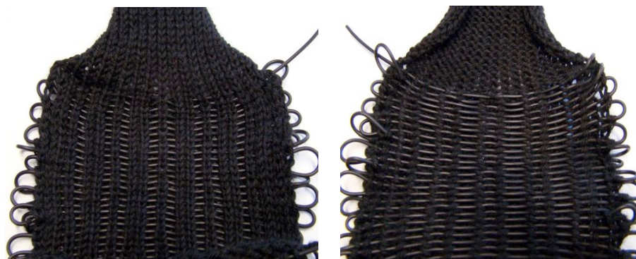
Figure IV: Sensor laid in every course with 100% wool, single bed looping and deformation as a result of drag front face and back
