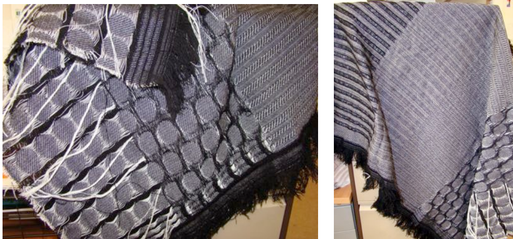
Figure VII: Large woven sample with float constructed channels
