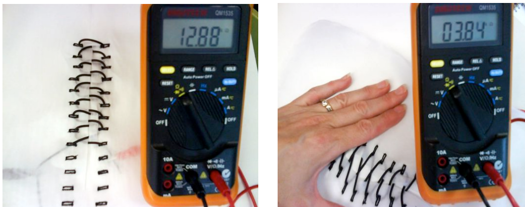
Figure XIII: Reducing resistivity with laced sample
